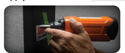
Carefully position the tool perpendicular to the work surface and guide the industrial fastener into the center of the attachment hole. Use a magnet or tape to temporarily hold the nameplate during fastening.
