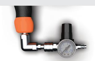
Start with 50PSI for fastening to aluminum, 60PSI for fastening to steel and 70PSI for cast iron. Raise PSI as needed.
