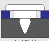
**Just Right**The attachment is secure and the locking groove is filled.
