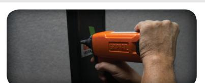
Depress the drive into the tool, then activate the trigger. (Always use both hands to hold the tool firmly in place.)
