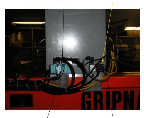
DRIVE VALVE P/N 44240 CORD SET P/N 51227 SHC SCREW #8-32 X 1" P/N 60159 NUT ESN #8-32
