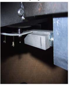
The sensor cables, shown below, contain two (2) light emitting diodes (LED's). The GREEN indicates the power is ON. The YELLOW indicates the sensor is activated by its target. This will help troubleshooting in the event a mis-adjustment or other service requirement.
