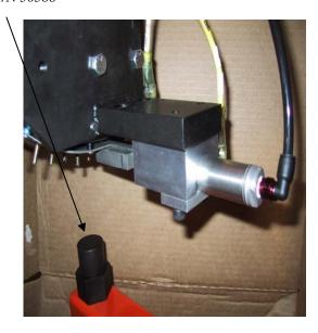
The transfer block fits into the track for easy alignment.
