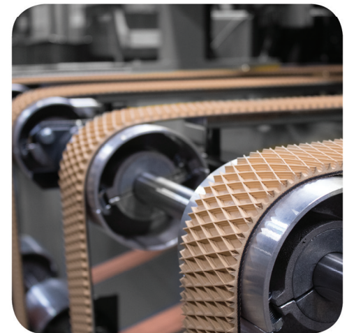
Magnetic Fabric Belts located below the carriage move the ductwork at 50 feet per minute.
