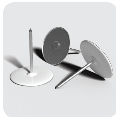
A Cupped Head Weld pin by GRIPNAIL is available with dielectric coating on the underside of the cap to prevent electrical contact with foil faced insulation.
